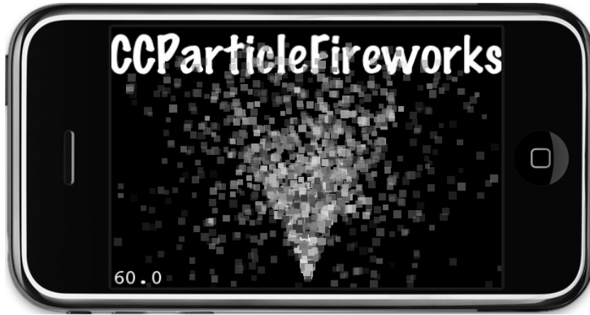
Figure 9-3. If your example particle effects, like this CCParticleFireworks , display huge, square particles, you forgot to add the fire.png image to your Xcode project
