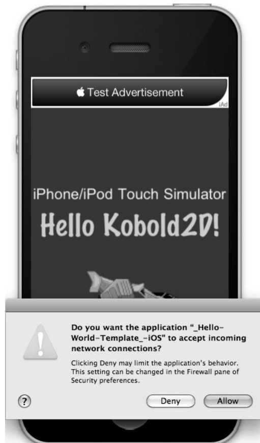
Figure 16-4. Network connection warning caused by iSimulate
