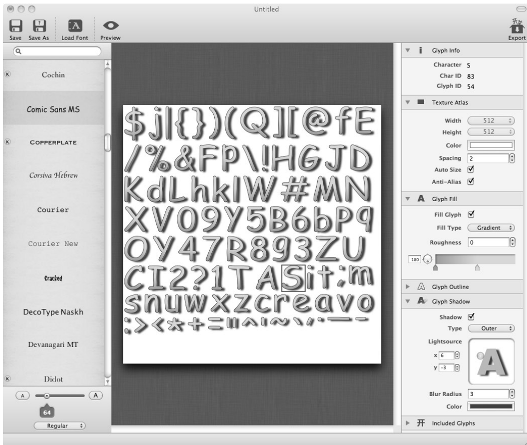
Figure 4-7. Glyph Designer lets you create bitmap fonts from any TrueType font and can export FNT and PNG files compatible with the CCLabelBMFont class of cocos2d
