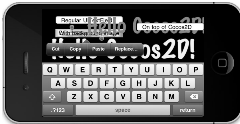
Figure 15-3. UIKit views on top and behind the cocos2d view, with input enabled for all of them
